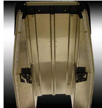
View of Firecat/Sabercat Tunnel
